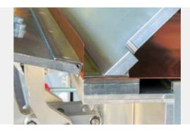
Turn metal sheet, carry out measurement 2, fold 145°
