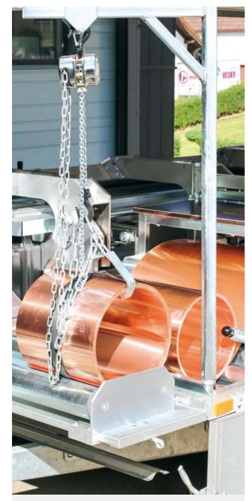
Lift and second uncoiling device
