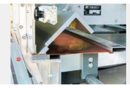
Carry out measurement 2, crimp with KNOLL profiling head
