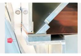
Turn metal sheet, carry out measurement 1, fold 180°
