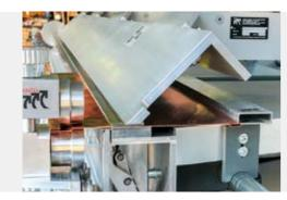
KNOLL hook-in panel is attached with fasteners. The hook-in panel can be placed with shadow gap or as rib on the other side.
