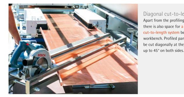
Diagonal cut-to-length system Apart from the profiling machine, there is also space for a diagonal cut-to-length system below the workbench. Profiled panels here can be cut diagonally at the right angle
