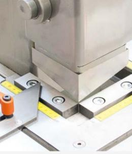
Notches  $90^{\circ}$ ,  $100 \times 100 \text{ mm}$ The metal sheet cut-out can be enlarged by resetting.
