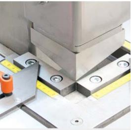
Notches 90°,  $100 \times 100 \text{ mm}$ The metal sheet cut-out can be enlarged by resetting.
