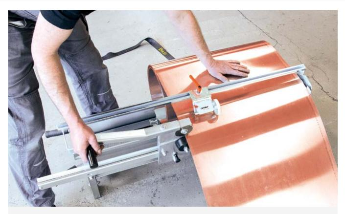
Transportation assistant and uncoiling device: the KNOLL Kuli The original KNOLL Kuli for the picking up, transportation, uncoiling and accurate cutting of metal coils. Your ergonomic helper for the workshop and the construction site.
