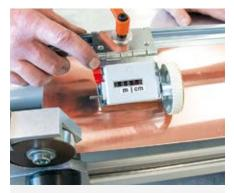
Length measuring device You can cut your metal sheet absolutely precisely with the Kuli shears and the length measuring device.
