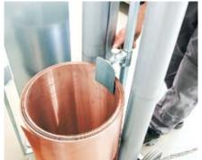
Coil holder/ coil rail The coil holder is particularly indispensable for the transportation of small coils. An exact infeed of the coil, e.g. to the profiling device, is achieved with the lateral coil rail.
